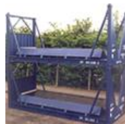
Figure 3.57 – Open steel coil carrier
