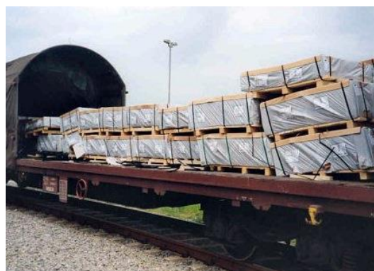
Figure 1.7 – Loose packages on rail wagon
