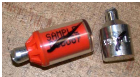
Figure 9.32 Cut bolt seals – head
