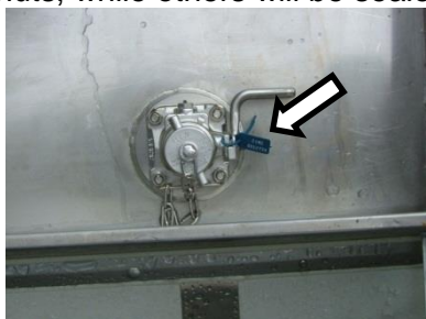
Figure 9.16 Top valve seal
