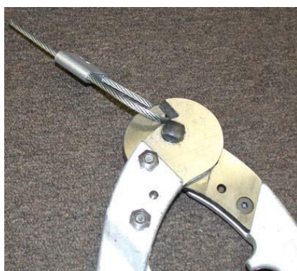
Figure 9.28 Cutters for cable seal
