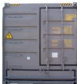
Figure 3.44 – Letterbox type hatch in fixed rear end
