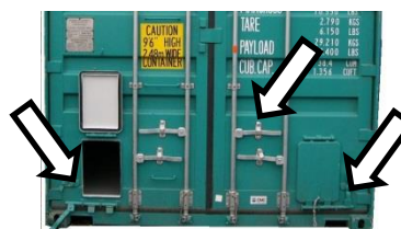
Figure 9.12 Dry bulk discharge hatch (rear)
