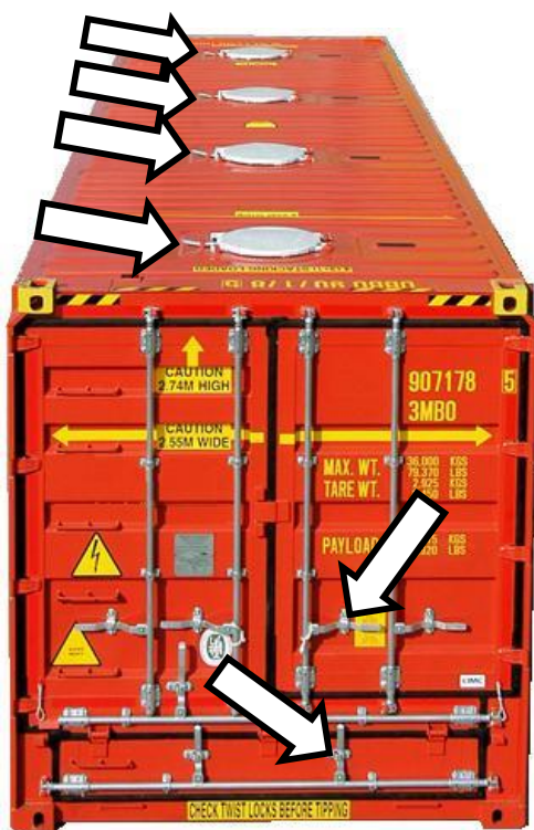
Figure 9.10 Dry bulk sealing points
