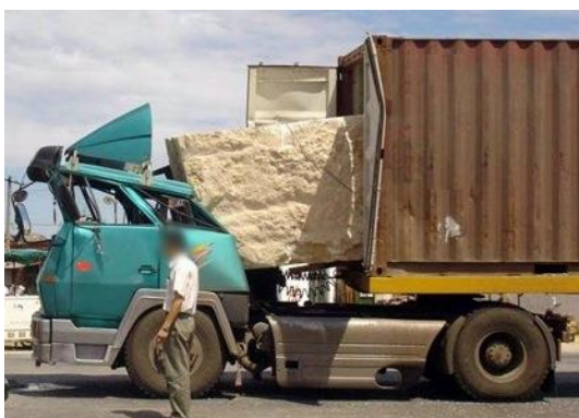
Figure 1.1 – Lack of longitudinal securing
