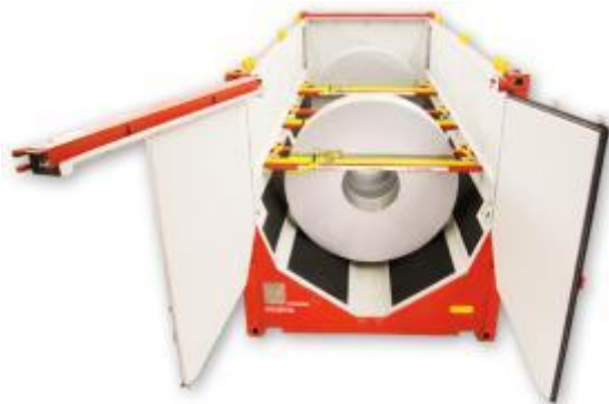
Figure 3.24 – 20-foot coil carrier
