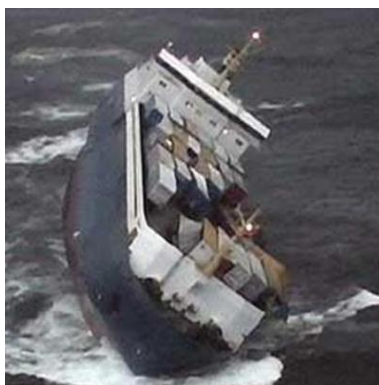
Figure 1.5 – Heavily listing ship after cargo has shifted
