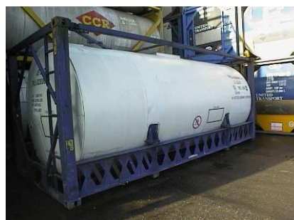
Figure 3.37 – 25,000 l frame tank
