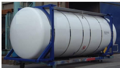
Figure 3.68 – Swap tank showing exposed ends
