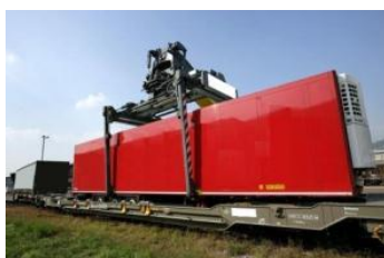
Figure 3.87 – Trailer1 loading using grapple arms
