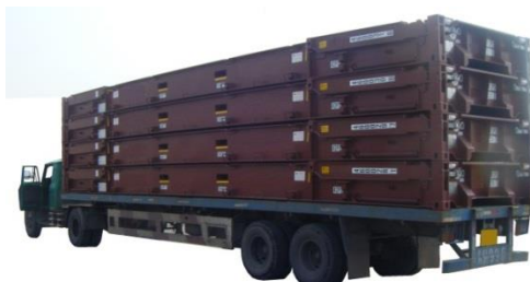
Figure 3.52 – Stack of 40-foot folding end flatracks
