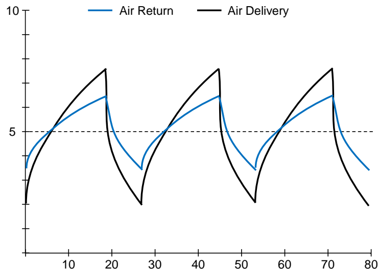
Figure 8.14 Variations of air temperature under thermostatic control
