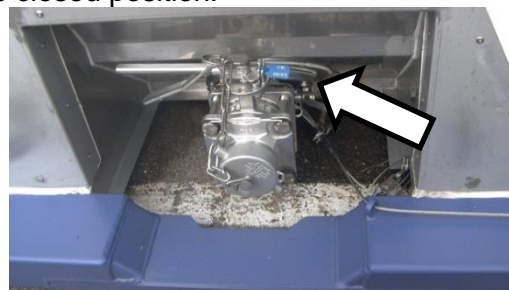
Figure 9.17 Discharge valve seal
