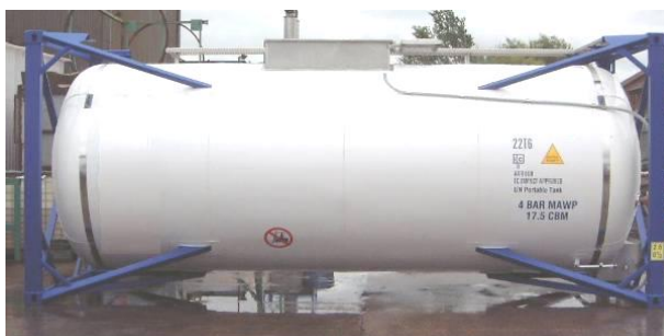
Figure 3.38 – Beam tank no top rail
