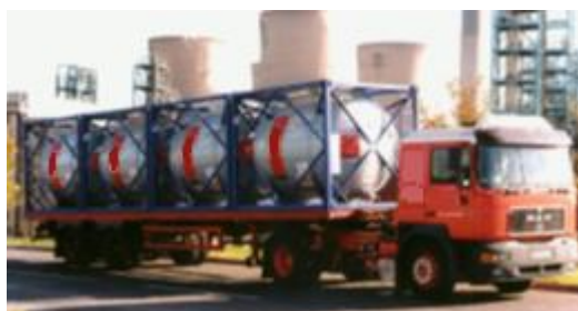
Figure 3.40 – Four 10-foot ISO beam tanks
