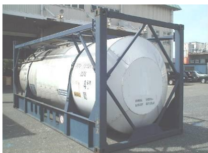
Figure 3.36 – 20,000 l frame tank
