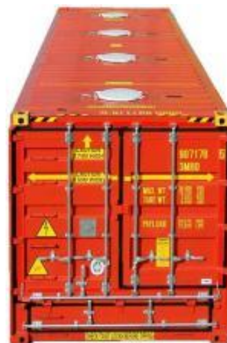
Figure 3.42 30-foot dry bulk box container
