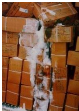
Figure 1.12 – Ice from leak in door gasket
