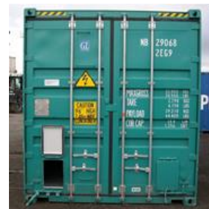
Figure 3.45 – Cat flap type hatch in rear doors
