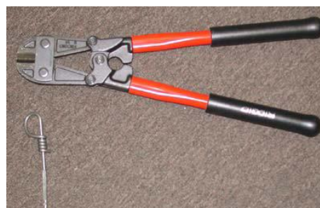
Figure 9.29 Cutters for twist seal
