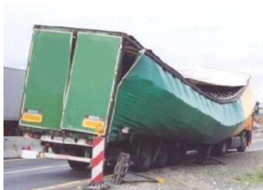
Figure 1.2 – Inadequate side wall strength
