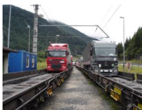
Figure 3.90 – Loading road vehicles
