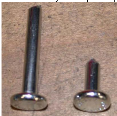
Figure 9.31 Cut bolt seal – stems
