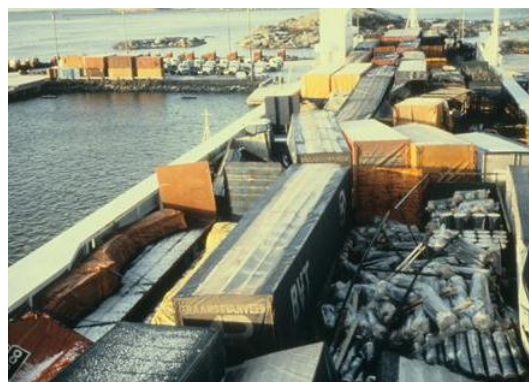
Figure 1.4 – Shifted cargo on a ro-ro deck
