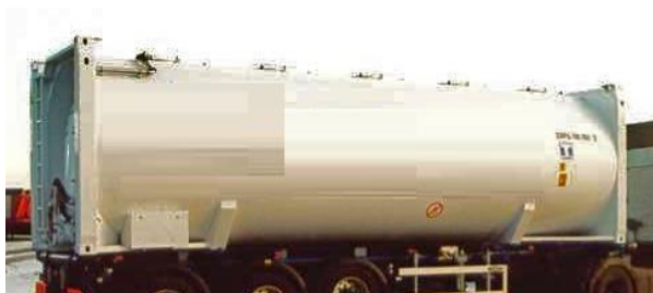
Figure 3.69 – 30-foot stackable swap tank for powder
