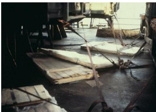
Figure 1.3 – Cargo breaking out of a trailer
