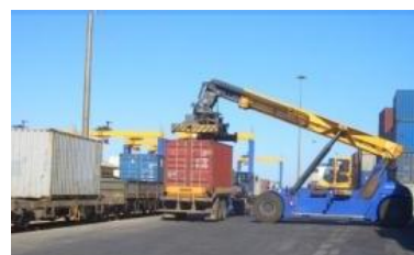
Figure 3.88 – Container loading using reach stacker
