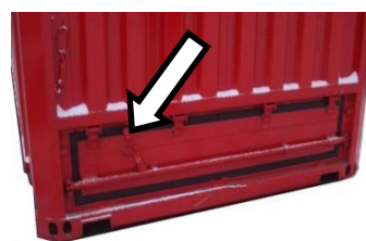
Figure 9.13 Dry bulk discharge hatch (front)
