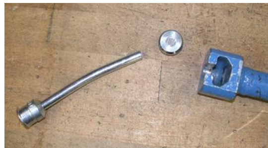
Figure 9.36 Rail car bolt seal and breaking tool
